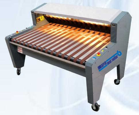
Production of 300 mats per hour (system and operator dependent)
